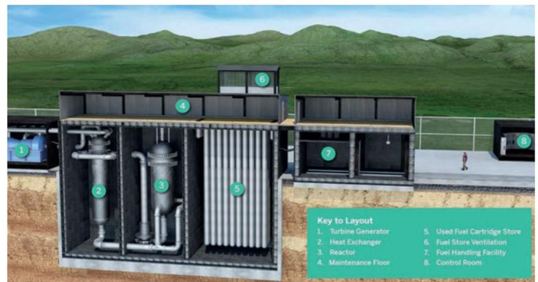
Figure 1 U-Battery Design (Source: www.u-battery.com/design-and-technology).
