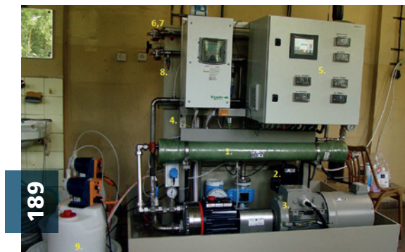
Overall view of the reverse osmosis pilot-plant at the Temelin NPP.
