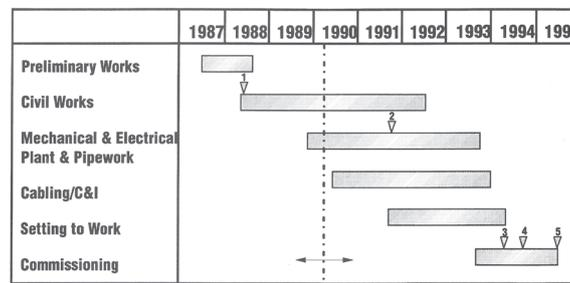
Fig. 1. Construction Programme. 1 First permanent structural concrete. 2 Start NSSS. 3 Hot functional testing. 4 Load fuel. 5 Full load.
