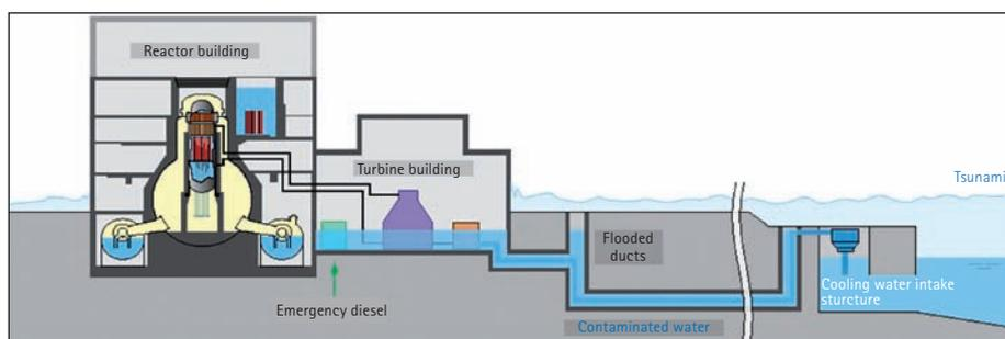
Fig. 1. Effects of the tsunami in the nuclear power plant Fukushima Daiichi.
