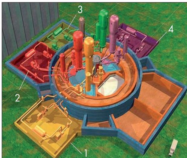
Fig. 8. EPR™ reactor: One section of the safety systems respectively is accommodated in each of the 4 safety buildings.
