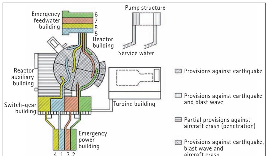
Fig. 5. Redundancy separation in German Konvoi plants.
